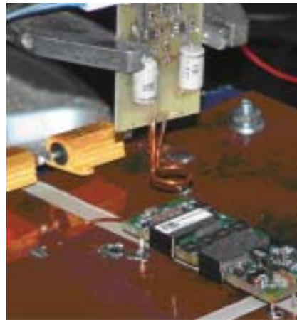
Figure 5 The intent is to place the pick-up loop 1 in. above the plane that would represent the surface of the motherboard if the converter were mounted in an appropriate through-hole design.
