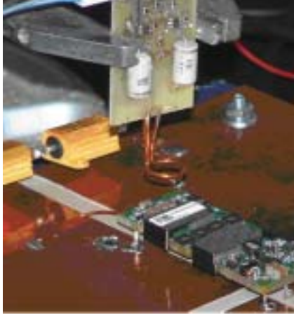
Figure 5 The intent is to place the pick-up loop 1 in. above the plane that would represent the surface of the motherboard if the converter were mounted in an appropriate through-hole design.
