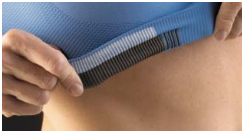
Figure 4 Textronics added a heart-monitor electrode to the lower band of a sports bra.
