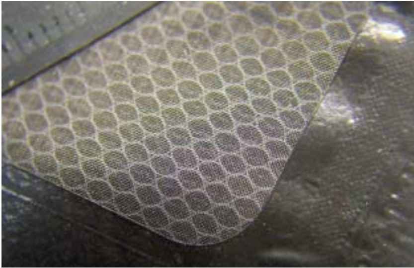
Figure 2 The ElekTex sensor contains a proprietary e-textile that senses pressure. It works by measuring voltage drop across the sensor surface.
