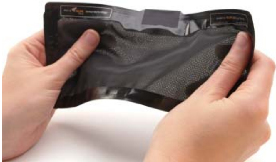
Figure 1 Users can roll, crumple, or fold Eleksen's textile pressure sensor, which finds use in keyboards for mobile electronics.
