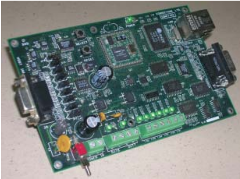
Figure 3 The ioNet embedded-device server module gives legacy industrial equipment or machines Web-based remote monitoring and control features.
