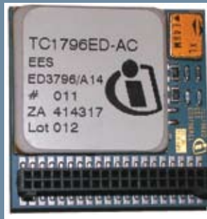
Figure B The TC1796ED emulation device has a USB port in the silicon.
