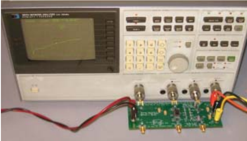
Figure 10 The gain- and phase-characterization pc board of the HP3577A network analyzer mounts directly on the front-panel connectors.
