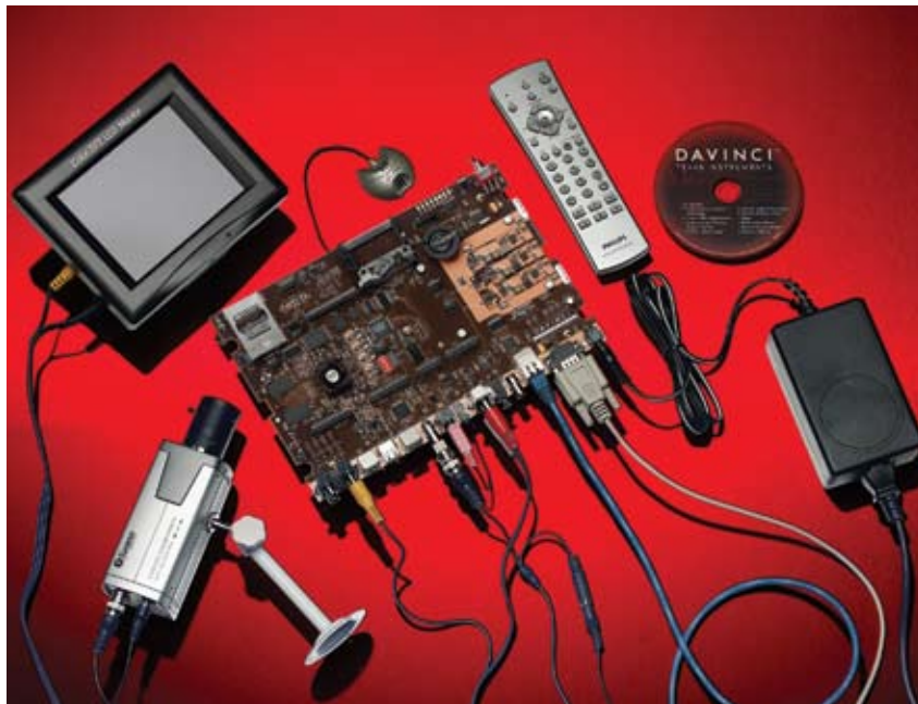
Figure 2 The Davinci evaluation module includes a camera, an LCD, an IR remote, speakers, and a hard-disk drive, as well as demonstration and development software.
