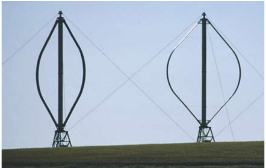
Figure 5 Vertical-axis Darrieus wind turbines can operate at higher efficiencies than their horizontal-axis peers; a simpler construction and immunity from wind-direction shifts are other advantages.
