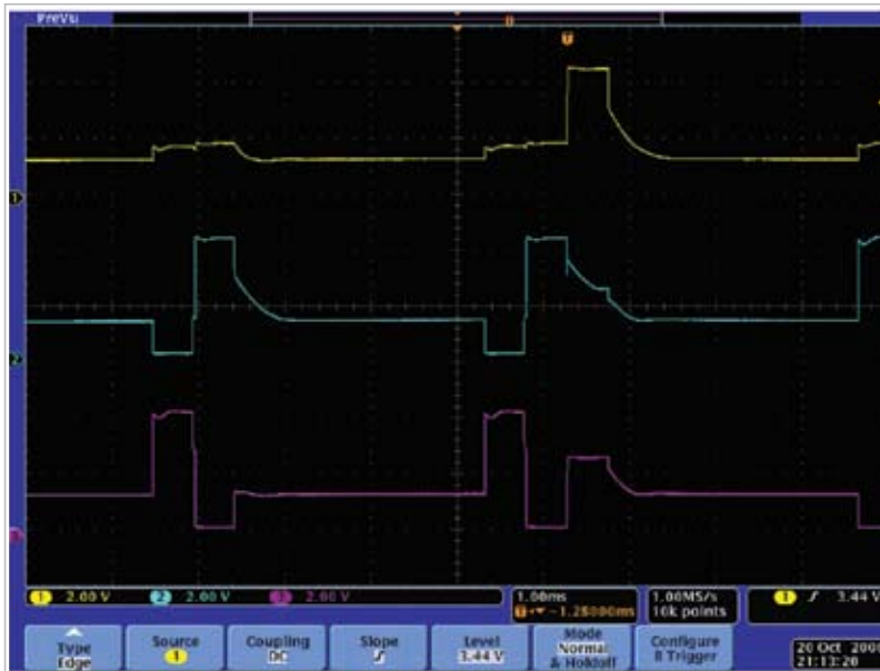
Figure 4 A digital oscilloscope captures the waveforms of GP0, GP1, and GP2 (upper to lower traces, respectively), which show a transition in the LED pattern from Case 7 to Case 8 (lines 62 and 63 in Listing led121.c.pdf).
