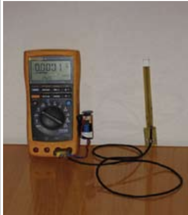
Figure 2 The digital multimeter's relative-change mode (RELΔ) displays a near-zero magnetic field reading and the sensor's nominal zero-field output voltage of 2.25V.
