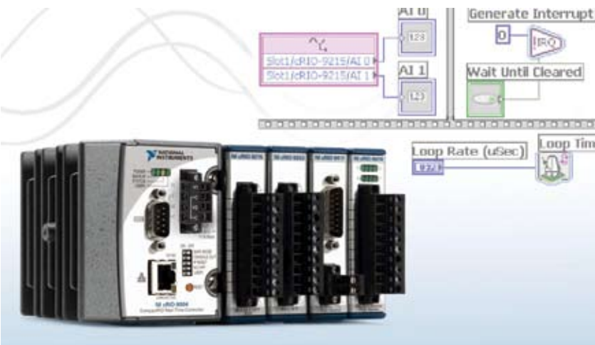
Figure 5 The CompactRIO system from National Instruments defines custom hardware circuitry using a reconfigurable FPGA and LabView graphical-development tools.
