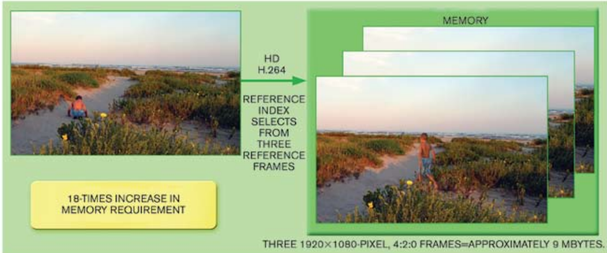
Figure 1 Decoding HD video requires significantly more memory, especially when you have employed advanced video codecs to compress it, than is necessary with SD video.
