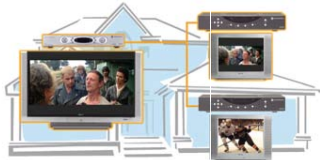
Figure 1 The Follow Me TV technology from Motorola will yield a distributed network of set-top boxes that allows consumers to view any live or stored programming anywhere in the home.
