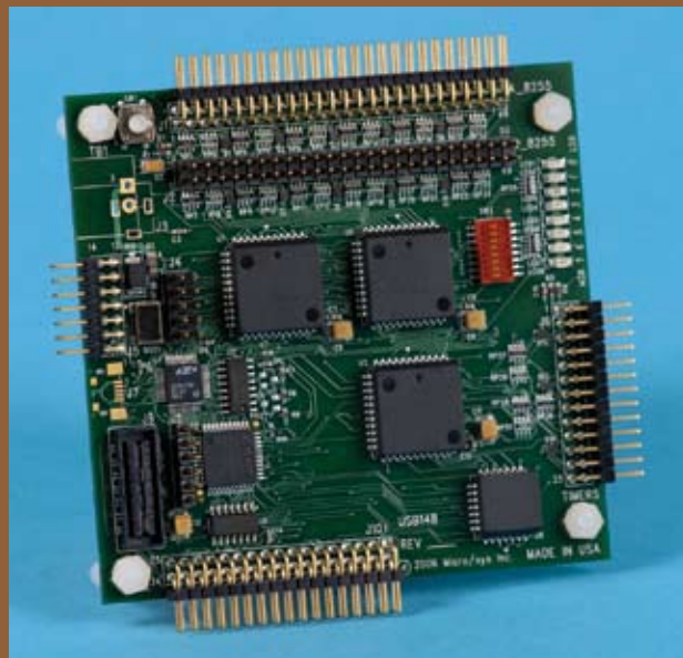
Figure A Although the industry has not yet approved it as a standard, the StackableUSB I/O module from Micro/sys includes 48 digital TTL I/O lines plus three timer/counters.
