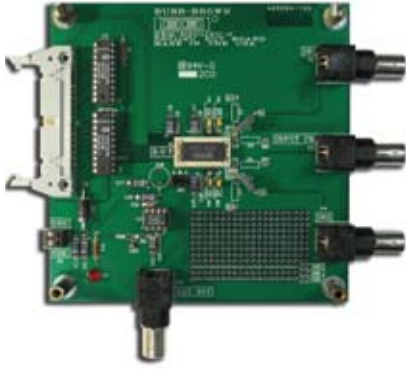
Figure 10 You can use this evaluation board for the DDC112 to measure femtoamperes of current. The DDC114 is even more sensitive (courtesy Texas Instruments).
