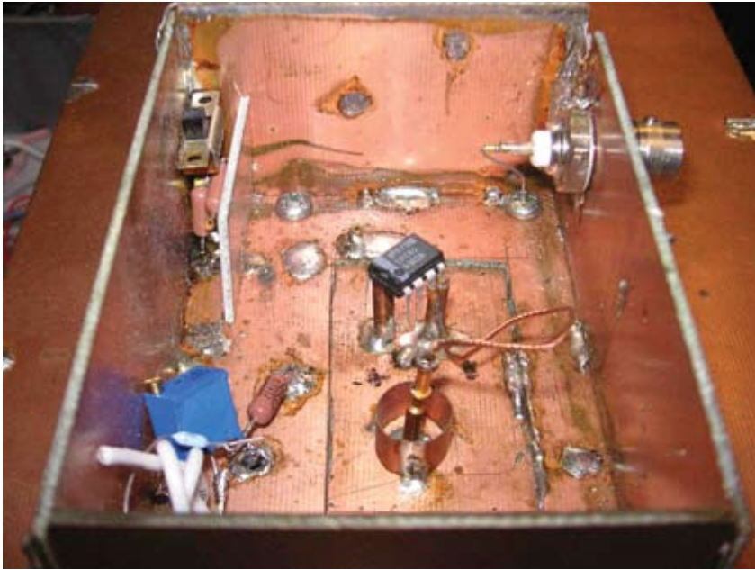
Figure 7 This configuration mounts the DUT on long standoffs that do not touch the PCB. Copper-clad boards serve as shielding (courtesy National Semiconductor).
