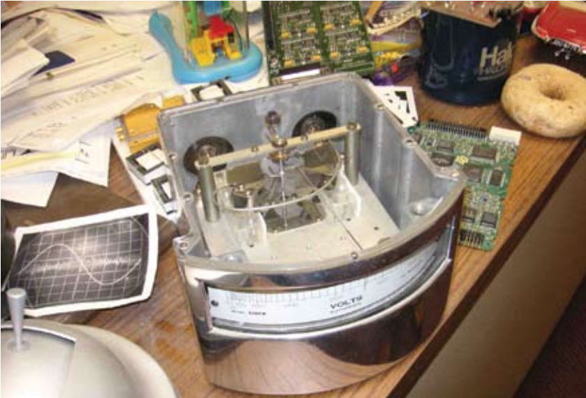
Figure A A rare class of analog meters uses electrostatic force. The plastic cover is for display. Rubbing the cover with your hand causes a triboelectric effect that pegs the needle (courtesy Jim Williams).
