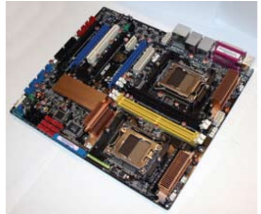
Figure 1 AMD's Quad FX system (a), containing two dual-core, 3-GHz CPUs (b), provides a speedy and flexible platform for benchmarking various external-storage options.
