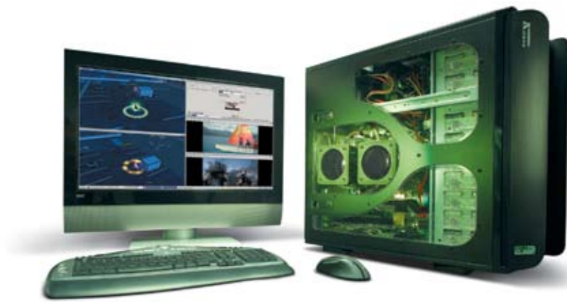
Figure 1 AMD's Quad FX system (a), containing two dual-core, 3-GHz CPUs (b), provides a speedy and flexible platform for benchmarking various external-storage options.
