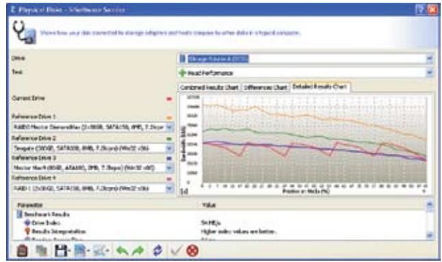
Figure 3 Single-drive- (a) and multidrive-concatenated (b) configurations both reveal varying data-transfer rates across a hard drive's platter.
