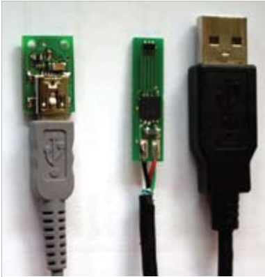
Figure 3 Two sample circuits (left and center) are smaller than a USB Type A plug (right).
