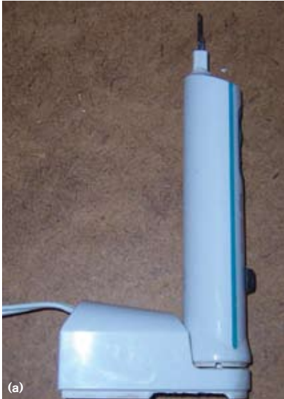
Figure 1 In this rechargeable electric toothbrush, no conductive contact occurs between the toothbrush holder and the charging unit. Energy transfer takes place through inductive coupling (a). This cutaway of the encapsulated base shows the primary winding of the transformer, with a ferrous rod pushing into the key that the toothbrush unit fits onto. Precise alignment is necessary to maximize the coupling between the two windings (b).
