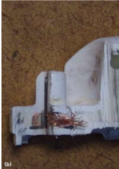
Figure 1 In this rechargeable electric toothbrush, no conductive contact occurs between the toothbrush holder and the charging unit. Energy transfer takes place through inductive coupling (a). This cutaway of the encapsulated base shows the primary winding of the transformer, with a ferrous rod pushing into the key that the toothbrush unit fits onto. Precise alignment is necessary to maximize the coupling between the two windings (b).
