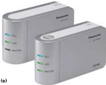
Figure 2 Power-line adapters include Netgear's 14-Mbps XE102 (a), Aztech Systems' 85-Mbps HL105E (b), and a triumvirate of 200-Mbps challengers: Linksys' HomePlug AV-based PLE200 (c), Netgear's DS2-based HDX101 (d), and Panasonic's BL-PA100 (e).
