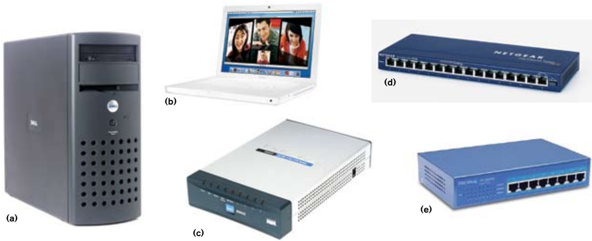
Figure A An owner-upgraded Dell PowerEdge 400SC (a) and wireless-updated Apple MacBook (b) were the endpoints for the lperf testing. A Linksys RV042 router (c), Netgear FS116 10/100 switch (d), and Trendnet TEG-S80TXE 10/100/1000 switch (e) acted as the network intermediaries.
