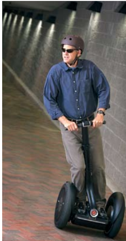
Figure 1 The Segway PT interface translates the leaning direction of the user into commands to move the PT in a direction (courtesy Segway).
