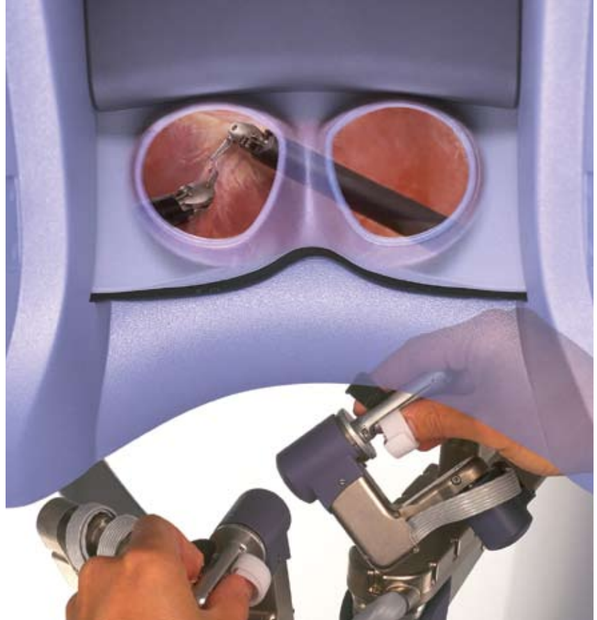
Figure 2 The da Vinci Surgical System combines two robotic systems, the masters and the EndoWrist Instruments, with a 3-D-vision system to enable surgeons to better perform complex laparoscopic surgical procedures (courtesy Intuitive Surgical).
