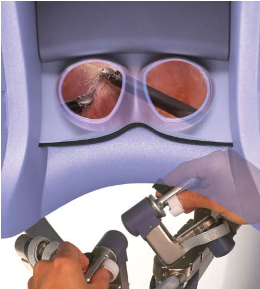
Figure 2 The da Vinci Surgical System combines two robotic systems, the masters and the EndoWrist Instruments, with a 3-D-vision system to enable surgeons to better perform complex laparoscopic surgical procedures (courtesy Intuitive Surgical).
