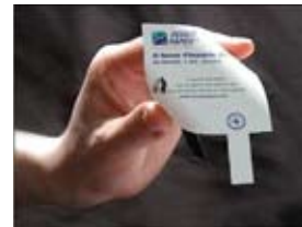
Figure 5 With layers of zinc and manganese dioxide to create the anode and cathode, Power Paper creates flexible and disposable printed batteries.
