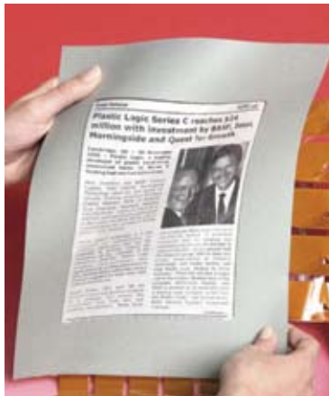
Figure 2 Electronic-paper displays employ an active-matrix backplane of printed transistors and conductors to produce portable electronic-reader products.
