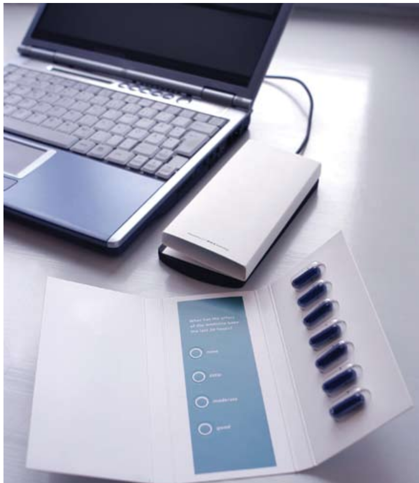
Figure 3 The Cypak intelligent-pharmaceutical-packaging system records medication use and is programmable to deliver patient reminders.
