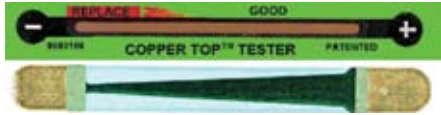
Figure 1 Interactive battery testers use conductive inks to form a resistive-heating element and temperature-responsive inks to indicate the charge (courtesy Duracell).
