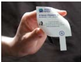
Figure 5 With layers of zinc and manganese dioxide to create the anode and cathode, Power Paper creates flexible and disposable printed batteries.
