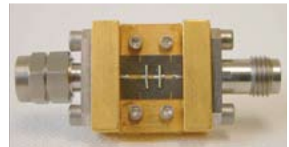
Figure 6 This test fixture has two small wires soldered across the transmission line connecting the two connectors. These wires add capacitance and show up as reduced impedance on a TDR plot (courtesy Picosecond Pulse Labs).
