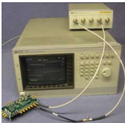
Figure 1 The HP 54120A mainframe, in concert with the 54121A test head, can take single-ended TDR and TDT measurements.
