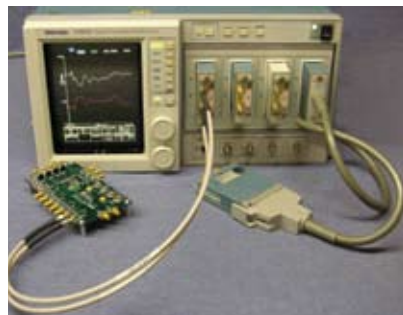
Figure 2 This Tektronix 11801B with four SD-24 TDR modules can take four pairs of differential TDR measurements. The scope traces show 10Ω of variance on PCB traces that should be 50Ω. The TDR shows how to improve this situation with layout and connector selection.
