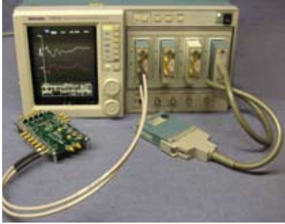
Figure 2 This Tektronix 11801B with four SD-24 TDR modules can take four pairs of differential TDR measurements. The scope traces show 10\Omega of variance on PCB traces that should be 50\Omega . The TDR shows how to improve this situation with layout and connector selection.
