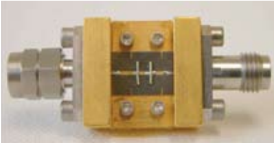
Figure 6 This test fixture has two small wires soldered across the transmission line connecting the two connectors. These wires add capacitance and show up as reduced impedance on a TDR plot (courtesy Picosecond Pulse Labs).
