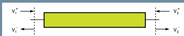
Figure A The S_{ij} parameter is the ratio of the reflected or transmitted wave at Port J to the incident wave at Port I.
