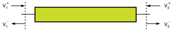
Figure A The S_{ij} parameter is the ratio of the reflected or transmitted wave at Port J to the incident wave at Port I.
