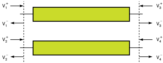
Figure B A four-port definition is more complicated, even though it is a direct extension of a two-port definition.
