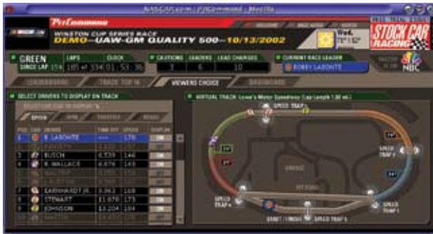
Figure 3 The NASCAR PitCommand feature allows fans to track race-car position, speed, and engine rpm in real time on their computers (above).
