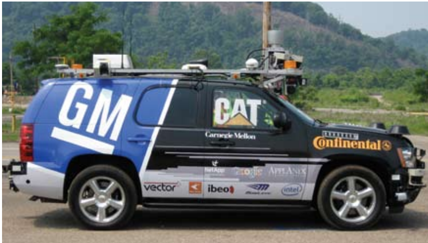
Figure 5 The Boss Chevy Tahoe sport-utility vehicle from Carnegie Mellon University will compete in the driverless DARPA Urban Challenge.
