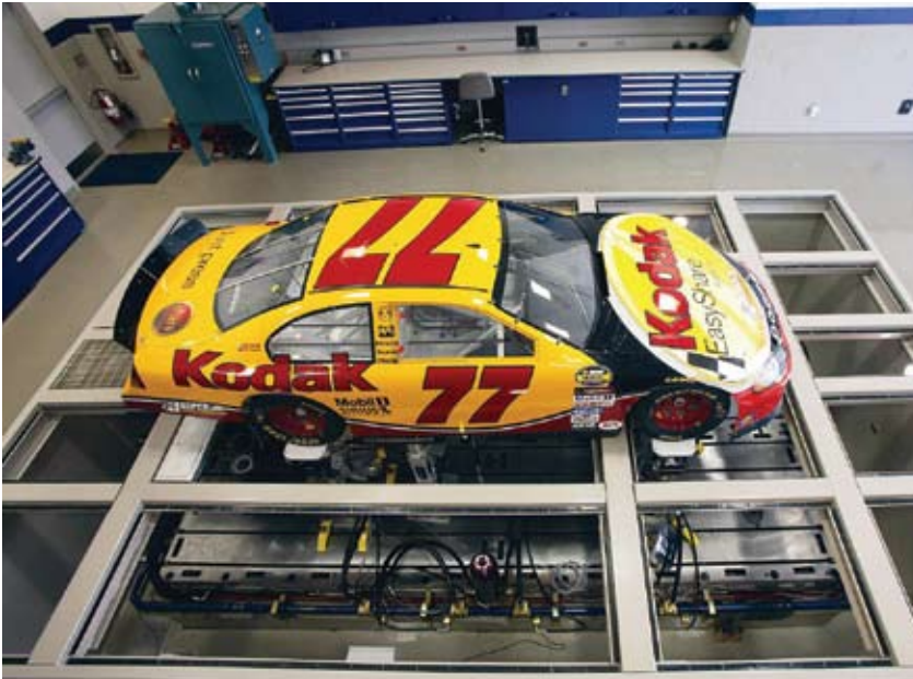
Figure 1 Penske Technology Group offers racing teams a shaker table and software to determine the best adjustments to vehicle-damping characteristics.
