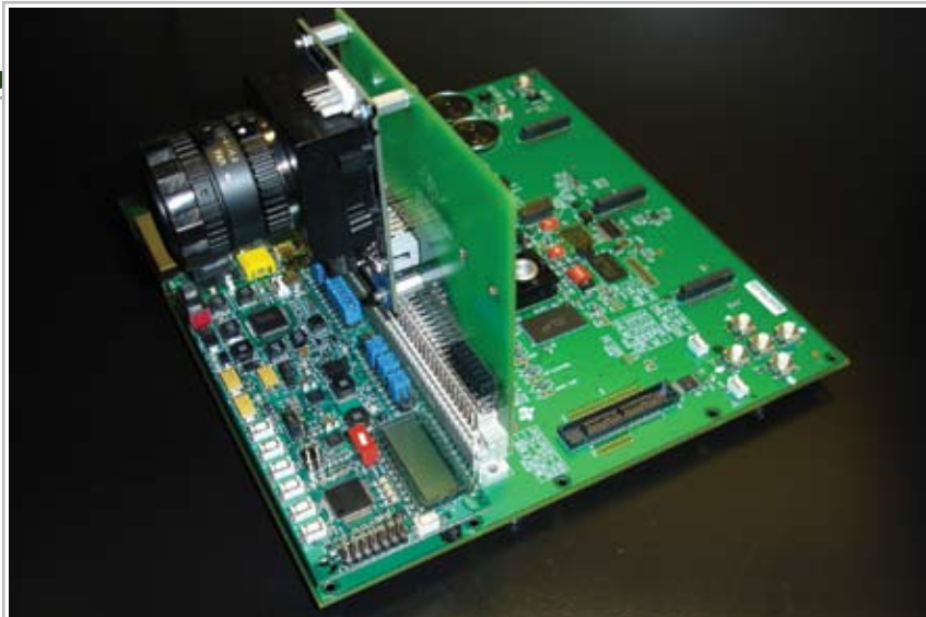
A Texas Instruments digital-camera reference design comes complete with a camera lens and a sensor.
