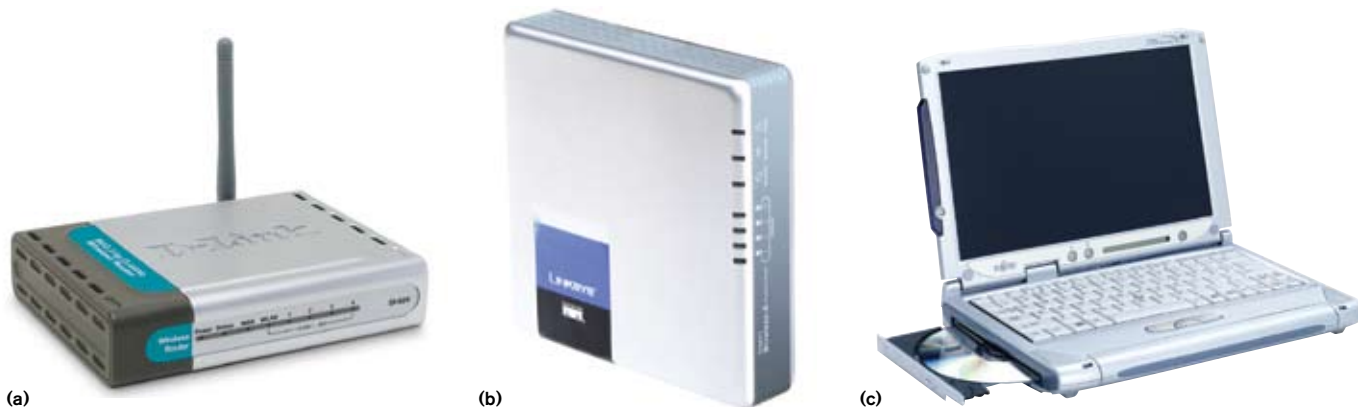
Figure 2 The DDNS client in D-Link's DI-524 appears to be nonfunctional (a), and the one in Linksys' WRT54GC is intolerant of lengthy network-initialization sequences (b). DynDNS' client software running on a Fujitsu Lifebook P-2110, however, operates as intended (c).
