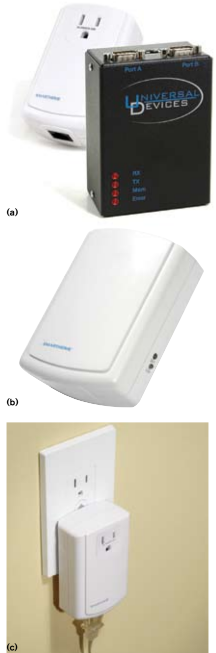
Figure 4 Smarthome's 2412S PowerLinc Modem is outlet-sensitive, at least in my setup, and it must be fully powered before you power up Universal Devices' ISY-26 to reliably manage it (a). The Smarthome 2443 access points aren't seemingly acting as the wireless phase couplers they're intended to be, although the reason why is unclear (b). Once I get my Insteon network to a more robust state, I'll advance it beyond its current humble implementation, switching two incandescent lamps via Smarthome 2856S3B on/off adapters (c).
