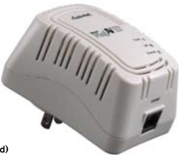
Figure 3 D-Link's DCS-1000W, being Java-based, is browser- and operating-system-agnostic but can't handle sun exposure (a). The 802.11b-based DCS-5300W (b) and 802.11g-supportive DCS-5300G (c) were unreliable over Wi-Fi, but Actiontec HomePlug AV adapters practically solved the connectivity problems (d).
