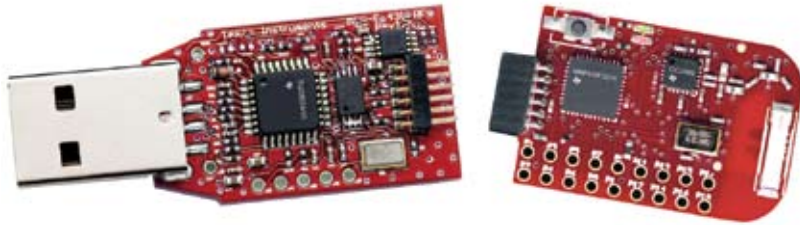
Figure 4 Texas Instruments' eZ430-RF2500 development tool was an extension-board candidate in part because of its modular approach to wireless communications.
