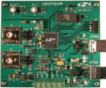
Figure 5 Silicon Labs' C8051F064EK evaluation kit was an extension-board candidate in part because of its dual ADC that could simultaneously take samples from two microphones.
