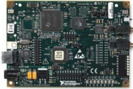
Figure 6 National Instruments' Speedy 33 signal-processing module includes dual integrated microphones and drivers and virtual instruments to work with the sampled data.
