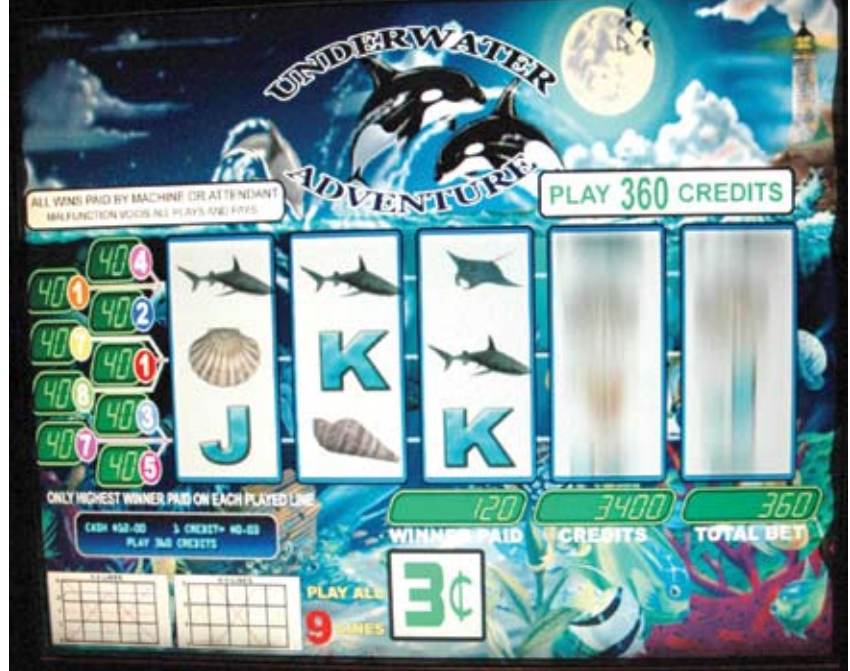
Figure 3 With two distinct screens sitting one behind the other to simulate depth, PureDepth’s MLD provides a realistic 3-D display.
