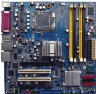
Figure 1 The iQ965-CI single-board computer combines Trusted Platform Module security technology and multimedia I/O for gaming-device applications.
