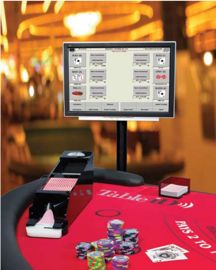
Figure 2 The Table iD system collects information from RFID chips and card readers to provide a snapshot of each player's gambling activity.
