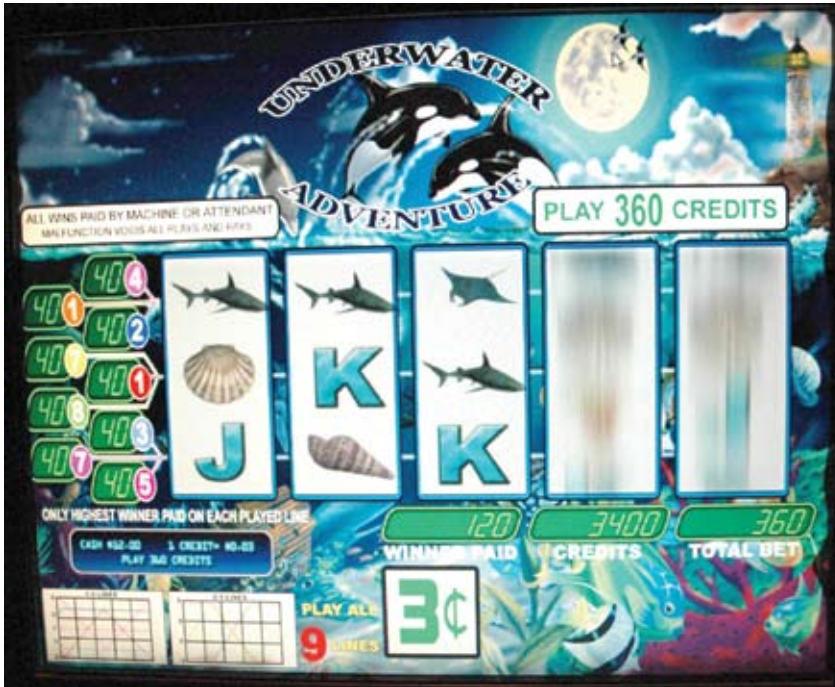
Figure 3 With two distinct screens sitting one behind the other to simulate depth, PureDepth's MLD provides a realistic 3-D display.
