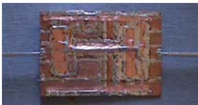
Figure 5 This copper-clad board has two antennas soldered to opposite sides of the same ground plane. When you operate circuits with fast edges on the board, the antennas radiate significant amounts of RF, even though they galvanically connect (courtesy Glen Dash).
