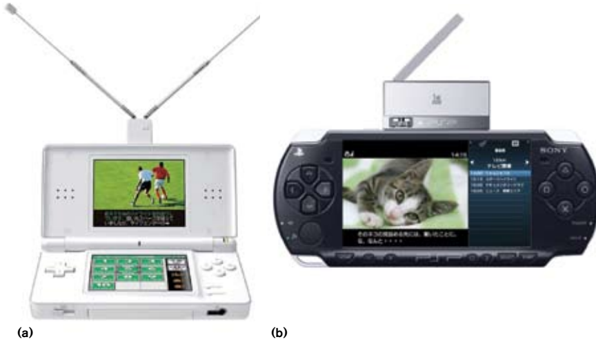
Figure 4 Nintendo's DS Lite (a) and Sony's second-generation PlayStation Portable (b) now support Japan's 1sec mobile-digital-video service, a subset of ISDB-T, through adapter add-ons.
