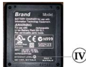
Figure 1 Although the Energy Star label on major appliances has a flashy Energy Star-compliance logo, the label on external power supplies is much smaller. Space constraints generally limit the designation to either III or IV, with III being the current spec, and IV indicating the tighter Version 2.0 proposed for 2008.
