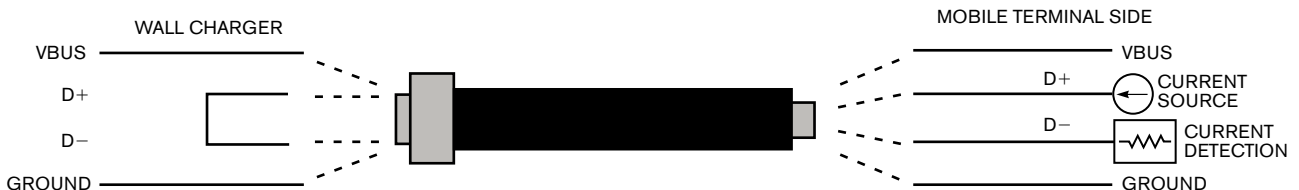
Figure 3 To control charging current, a new spec from the USB Implementers Forum calls for wall-mounted battery chargers to implement this design, which connects the USB connector's D+ and D- pins but does not otherwise connect them.
