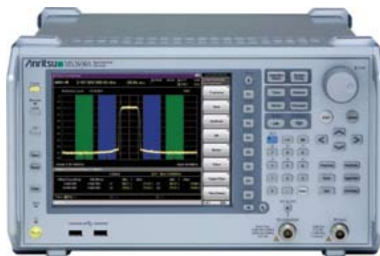
Anritsu M2690A/M2691A signal analyzers operate from 50 Hz to 6 GHz and can measure the transmitting power of mobile-WiMax devices.
